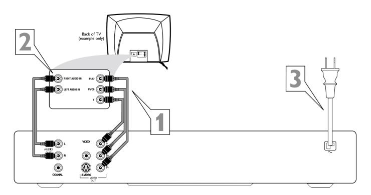
Connect the Player's green, blue, and red Y Pb Pr (VIDEO OUT) jacks to the corresponding COMPONENT VIDEO IN jacks on the TV. Use component video cable (not supplied).
